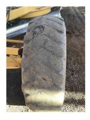
Make / Serial#Tread Depth in 1/32"% Life Recapped Recapped Cuts/ChunksTread Side Cuts SectionYokohama1545NOYESYES
