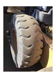
Make / Serial#Tread Depth in 1/32"% Life Recapped Recapped Cuts/ChunksTread Side Cuts Cuts/ChunksBridgestone515NOYESYES
